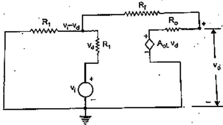
**Equivalent circuit of non-inverting amplifier using low-frequency model .**
