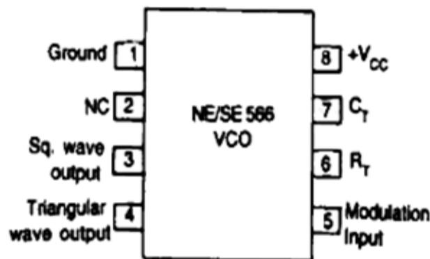
Figure 26 (a) Pin configuration
