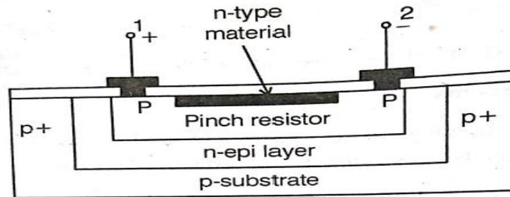
Fig 4.3.3 Pinched resistor
