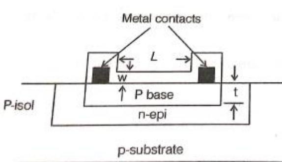
Fig 4.3.1 (a) Base resistor
