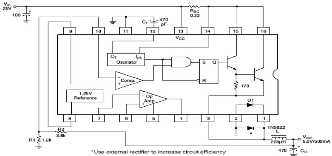
Figure 6. Step-Down Converter
