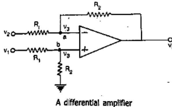
→  $V_1$  and  $V_2$  are the two input signals while  $V_0$  is the single ended output. Each signal is measured with respect to the ground.
