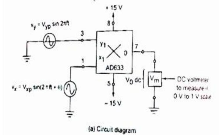
**Figure 44: Phase angle detector**
