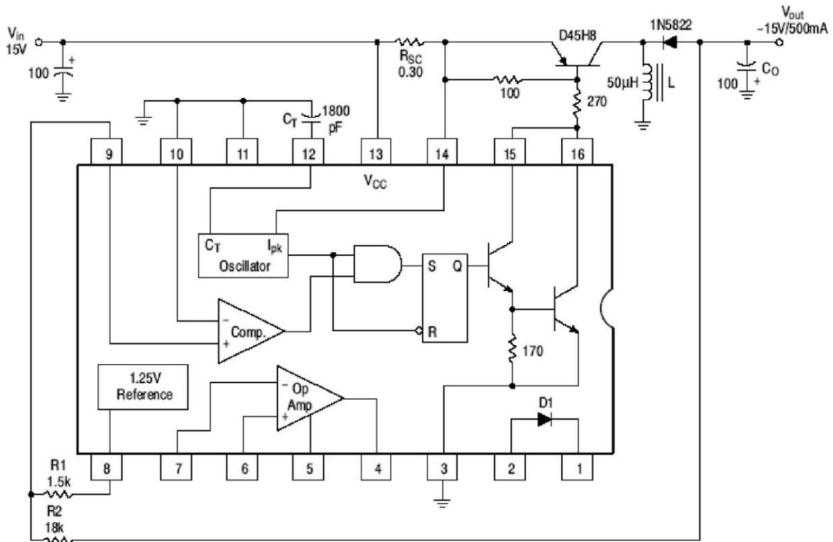
**Figure 17: Inverting switching regulator**
