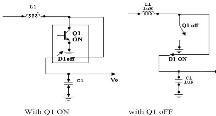
**(iii) Inverting Switching Regulator:**
