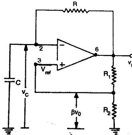
**Fig. 3.30 Simple op-amp square wave generator**
