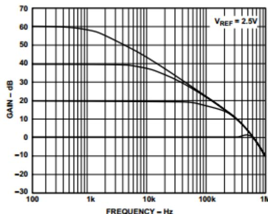
**Figure 2: AD623 Closed-Loop Gain vs. Frequency**
