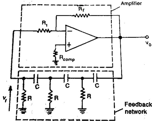
**Fig. 3.41 Phase Shift Oscillator**
