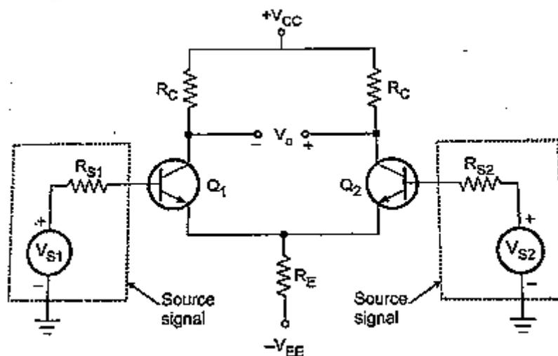
**Dual input, balanced output differential amplifier**
