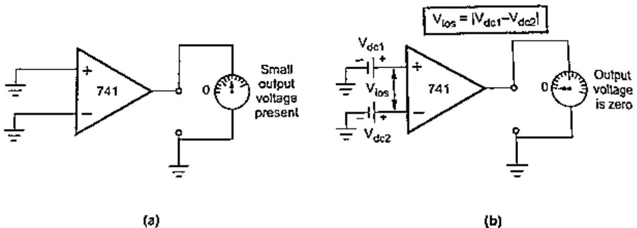
**Concept of input offset voltage**
