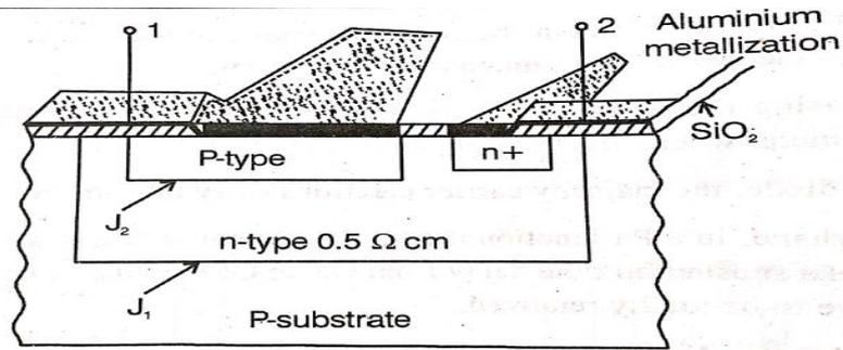
Fig 4.2.1 Junction capacitor
