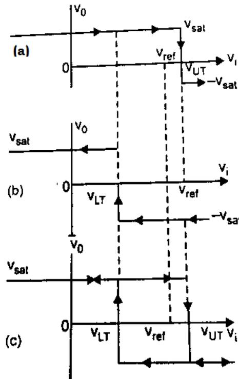
**Fig. 3.27 (a, b) Transfer characteristics for  $v_i$  increasing and  $v_i$  decreasing
