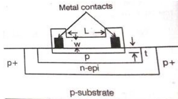
Fig 4.3.1 (b) Emitter resistor
