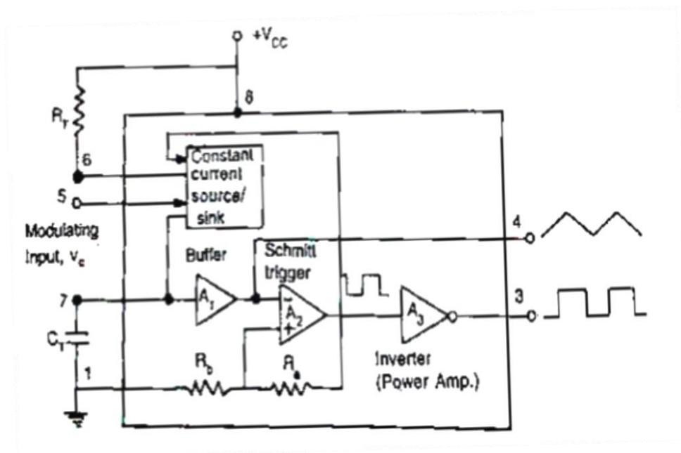
Figure 26(b): Block diagram
