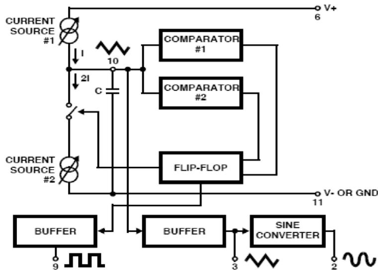
**Fig 19: Functional block diagram of Function generator**
