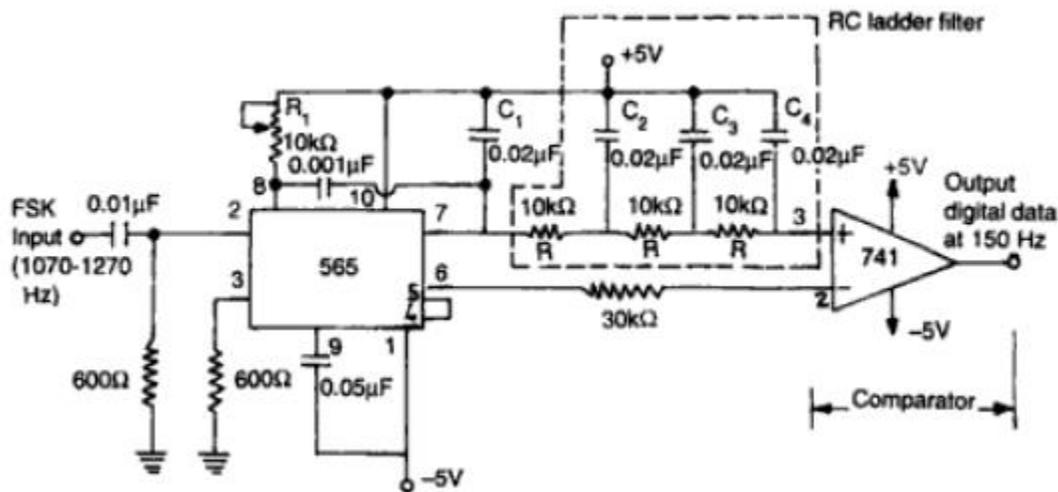
**Figure 32: FSK Demodulator**
