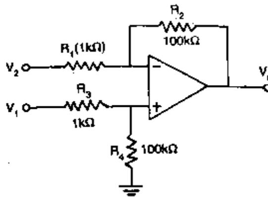
**Fig. 3.1 Differential amplifier using single op-amp**
