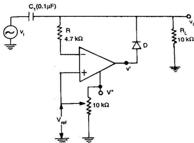
Fig. 3.48 Peak Clamper Circuit
