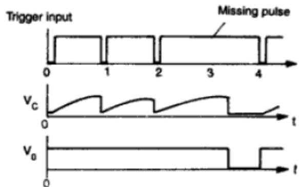
Figure 9: Output of missing pulse detector
