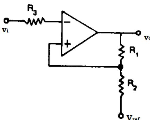
**Fig. 3.26 An inverting Schmitt trigger**
