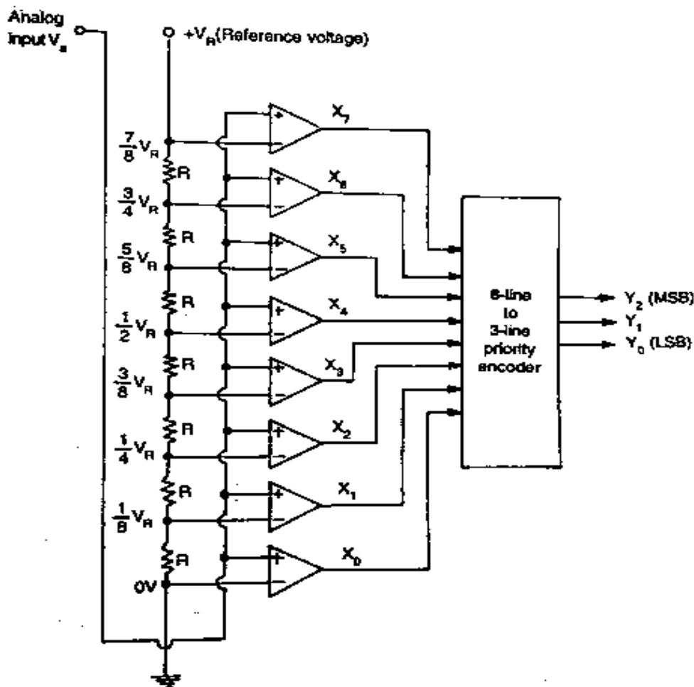
**Fig. 3.61 Flash type A/D Converter**
