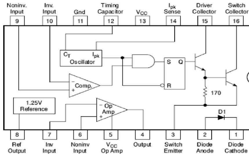
**Fig 13: Functional block diagram of  $\mu$ A78S40**
