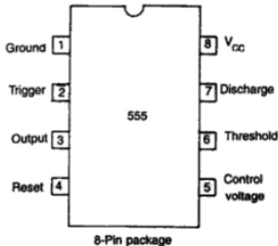
**Figure 1: Pin Diagram**
