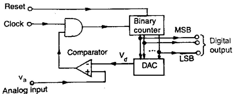
Fig. 3.64 Counter type A/D Converter
