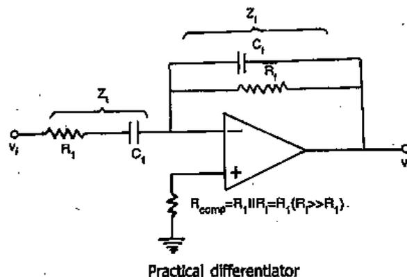
→ The transfer function for the circuit in Fig. is given by,
