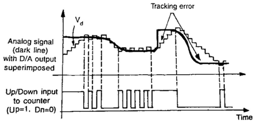
Fig. 3.66 Waveforms associated with tracking A/D Converter
