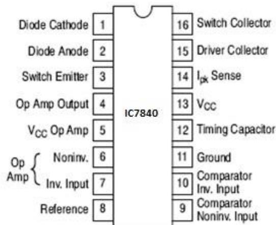
**Fig 14: Pin Diagram**
