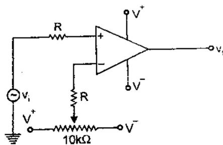
**Fig. 3.20 Practical Non-inverting comparator**
