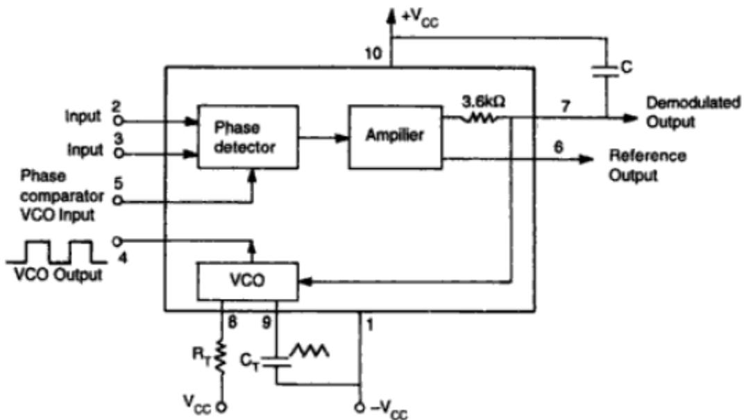
Figure 27 (b) NE/SE565 PLL block diagram
