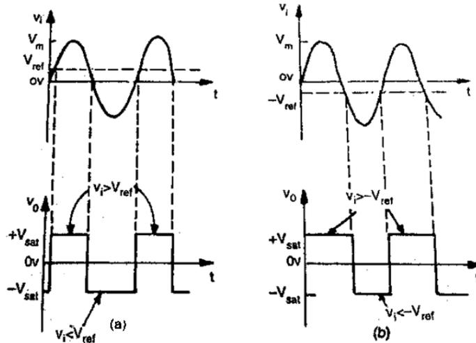
**8. Draw the input and output waveforms of inverting comparator if input is purely sinusoidal.**
