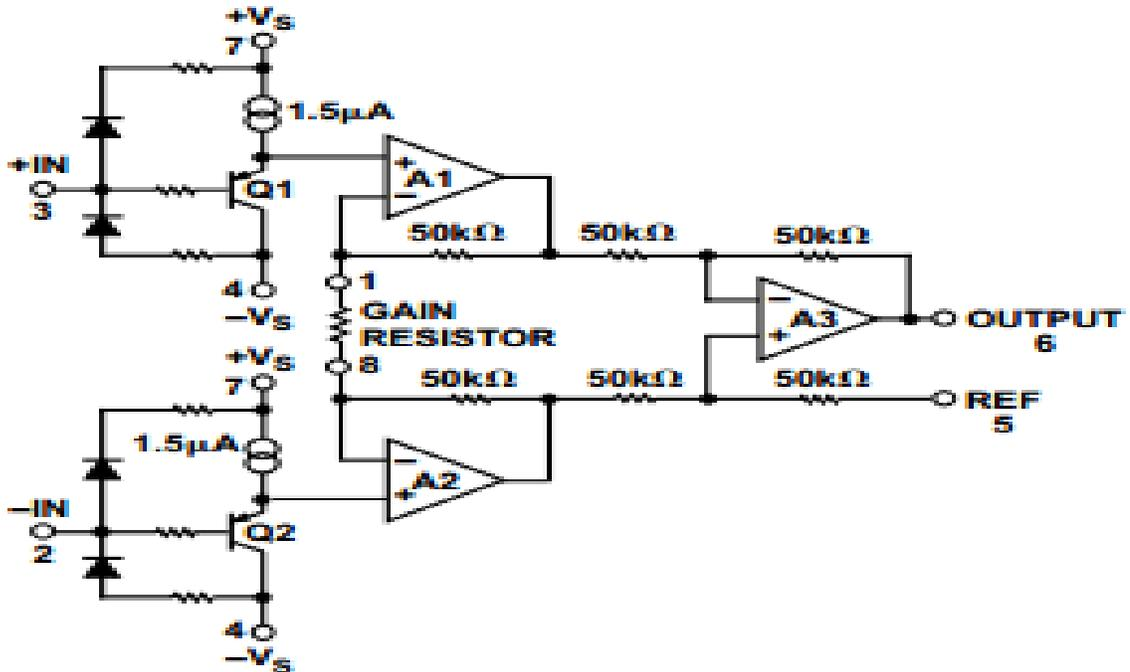
**Figure 1: AD623 Simplified Schematic**
