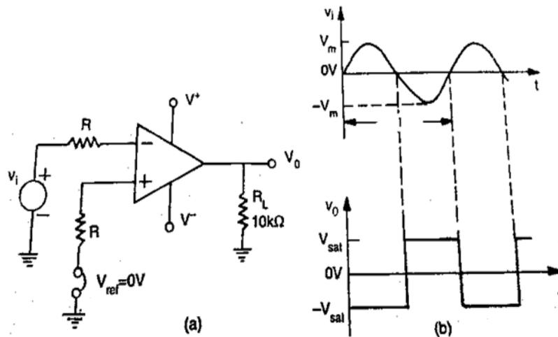
**Fig. 3.24 (a) Zero crossing detector (b) Input and Output Waveforms**
