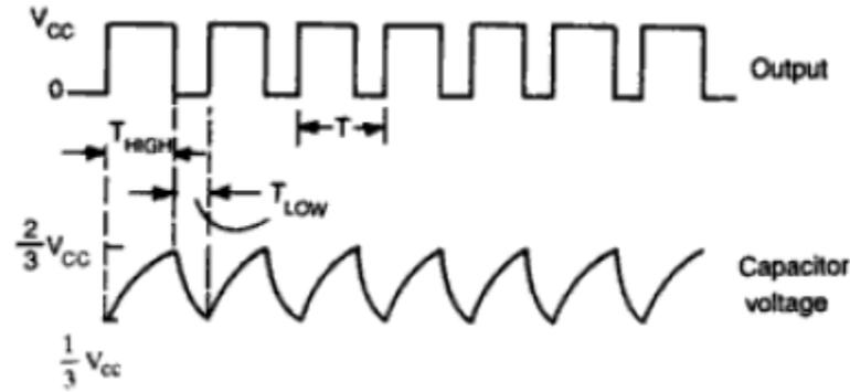
**Figure 17: Timing sequence of Astable multivibrator**
