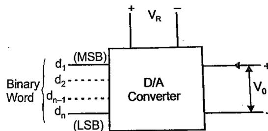
**Fig. 3.55 Schematic diagram of a DAC**
