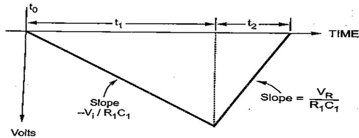
**Fig. 3.68 Integrated output waveform for the dual slope ADC**
