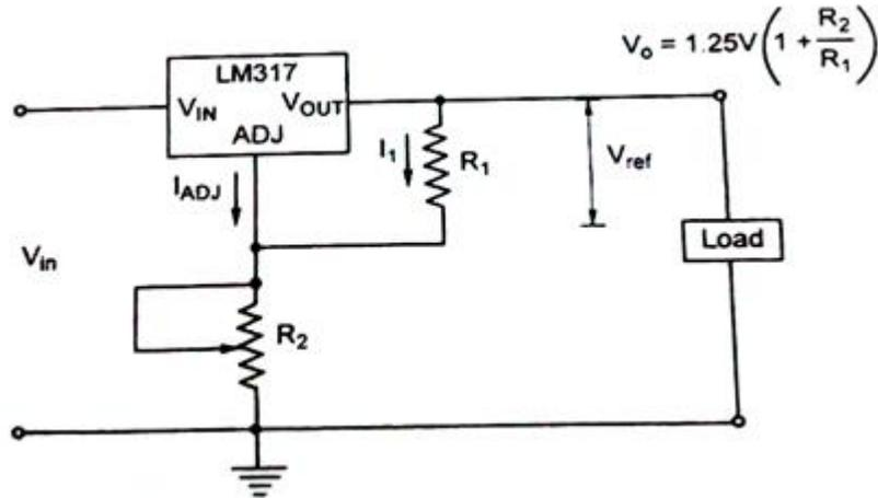
Figure 6: LM 317- Voltage regulator
