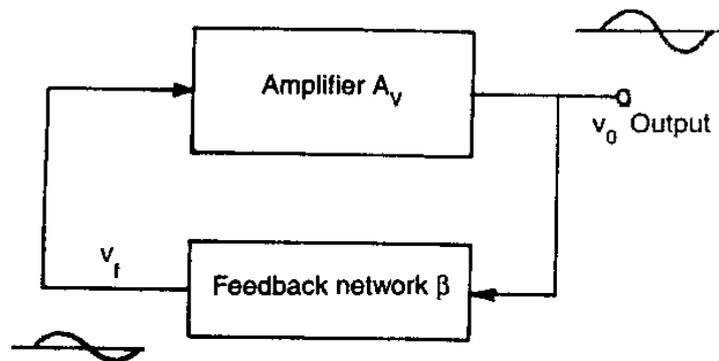
**Fig. 3.40 Block diagram of a feedback oscillator**
