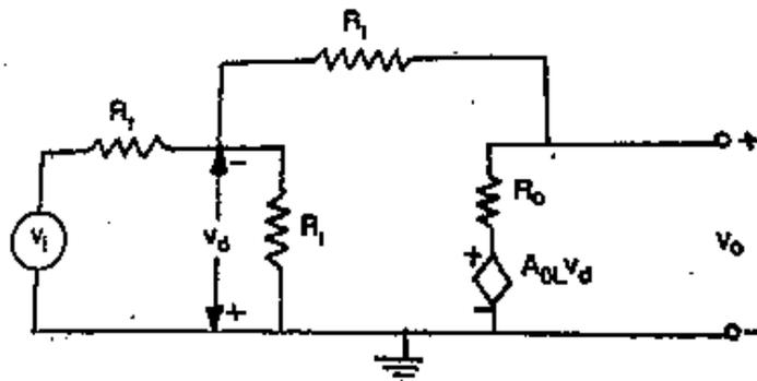
**Equivalent circuit of a practical op-amp inverting amplifier**
