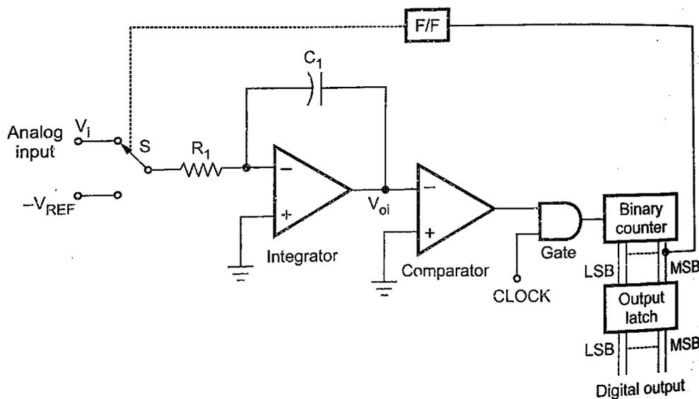
Fig. 3.67 Functional diagram of Dual Slope ADC
