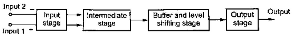
**Internal block schematic of an op-amp**
